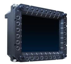
A PARTICULAR FOCUS OF THE COMPANY'S ACTIVITY IS THE DESIGN OF COCKPIT DISPLAYS BASED ON LCD PANELS. THESE PRODUCTS OPERATE IN SEVERE ENVIRONMENTS AND GUARANTEE SUNLIGHT READABLE IMAGE (UP TO 100,000 LUX).
