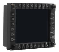
VIDEO MODULE VM-300 IS DESIGNED FOR DISPLAYING INFORMATION FROM AIRBORNE AVIATION CALCULATORS IN CONDITIONS OF DIRECT SUNLIGHT, SHARP TEMPERATURE AND PRESSURE DIFFERENCES, MECHANICAL OVERLOADS. ON THE FRONT PANEL THERE ARE 28 BACKLIT FUNCTION BUTTONS, 3 ENCODERS WITH PUSH FUNCTION, "DAY/NIGHT" MODE SWITCH, 2 PHOTO SENSORS.
