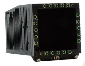
THE AVIATION VIDEO MONITOR IS DESIGNED FOR DISPLAYING VIDEO INFORMATION RECEIVED VIA ANALOG VGA INPUT FROM THE ONBOARD COMPUTER. DISTINCTIVE FEATURES OF THE PRODUCT ARE THE PRESENCE OF A FUNCTIONAL KEYBOARD, INFORMATION EXCHANGE WITH WHICH IS CARRIED OUT VIA ARINC-429 INTERFACE, MANUAL AND AUTOMATIC ADJUSTMENT OF IMAGE BRIGHTNESS, FORMATION OF INTERNAL TEST IMAGE.
